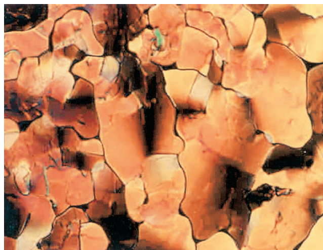
Figure 7. Mosaic texture observed for the SmX 2 phase at 121.6^{\circ}\text{C} , for 8OSO11SO8 cooled from the SmA phase using slides treated for homeotropic alignment.
